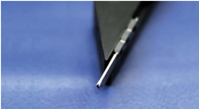
Tool to cut thin-walled parts off
