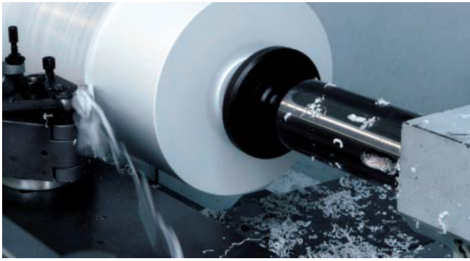
Continuous chip during lathe turning
