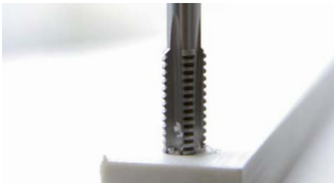
Thread cutting with a threading tap
