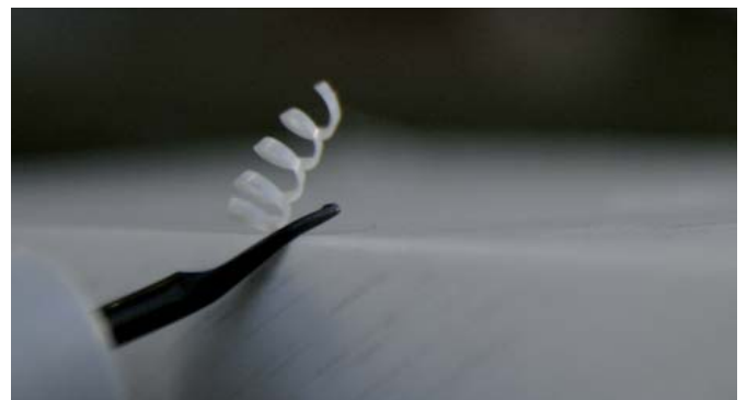
Burr removing using a burring blade
