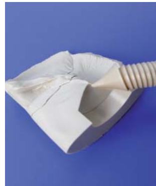
Rupture due to large chip removal
