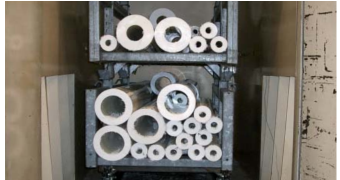
Annealing to reduce tensions
